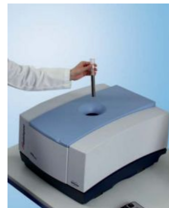
The tube to be inserted in the TD-NMR instrument including the sample
